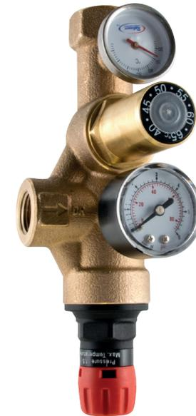
Designed to combine the functionality of a thermal balancing valve which regulates water within a hot water circulation system, with the functions of a pressure reducing valve which reduces a high inlet pressure to a lower outlet pressure.
